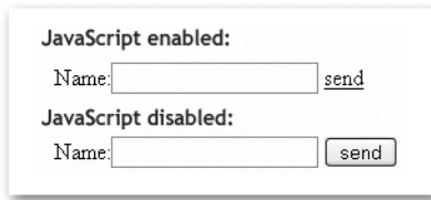
Figure 4-12. Depending on JavaScript availability, the user gets a link or a button to send the form.
