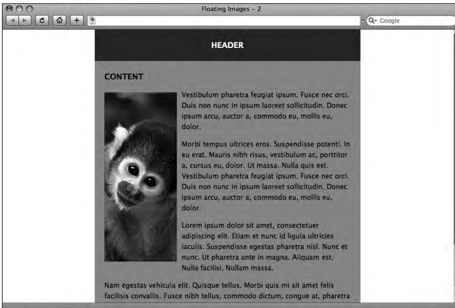
Figure 11-19. Applying a float: left; results in our image being removed from the normal document flow and the text wrapping around it.
