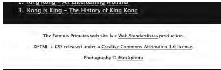
Figure 10-24. The a:link and a:visited pseudo-classes are now styled differently, set in the same color as the p elements in the footer.
