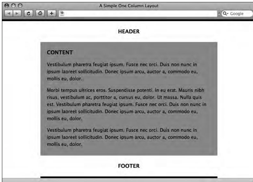
Figure 10-20. Note how the border at the top spans the entire width of the body, whereas the border at the bottom spans only the width of the container div .
