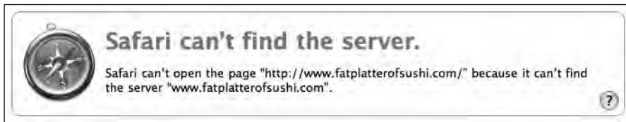
Figure 7-3. Our browser can't find the server www.fatplatterofsushi.com because the domain name hasn't yet propagated.
