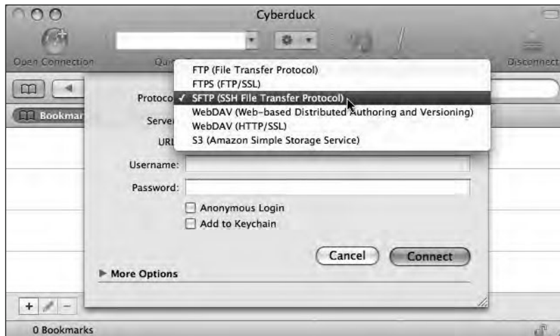
Figure 7-5. Cyberduck, like most file transfer applications, allows other, more secure protocols than FTP.
