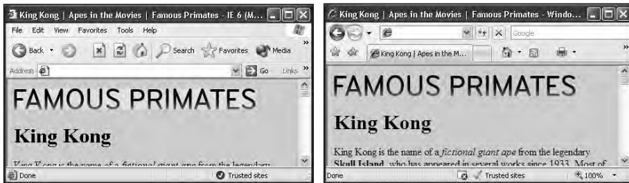
Figure 5-14. A PNG-24 with transparency rendered in Internet Explorer 6 and 7. In IE 6, on the left, the image background isn't transparent.
