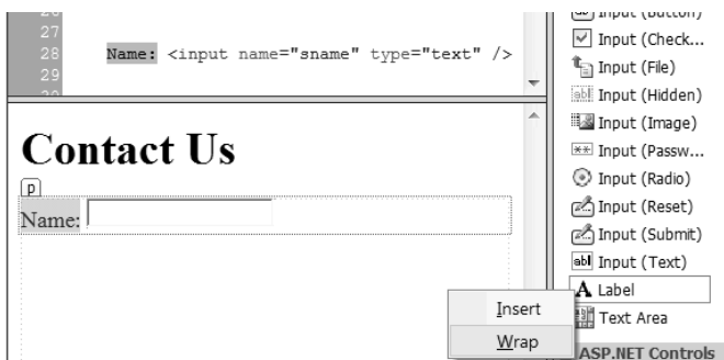
Figure 10-16. Highlighting the text and the form field will wrap the label around the selected items.
