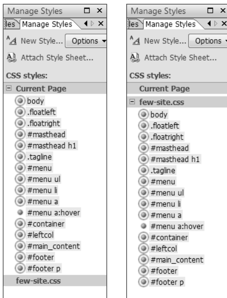
Figure 8-23. Move styles from the page to your external stylesheet by dragging between the sections.
