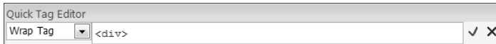
Figure 7-4. Using Wrap Tag will put your opening and closing <div> elements around the selection without having to go to Code view.
