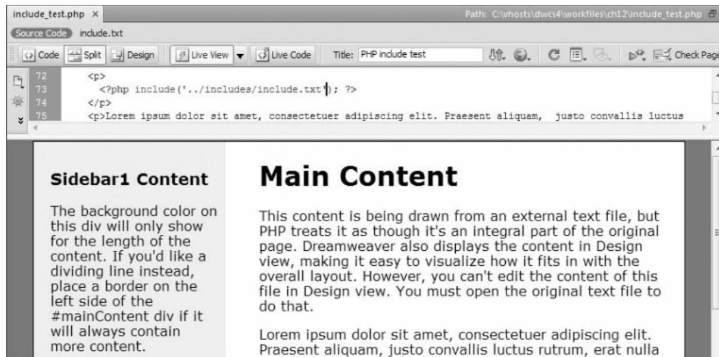
Figure 12-3. The include file is displayed correctly when a relative path is used.
