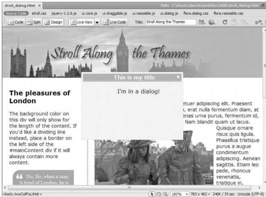
Figure 8-12. The default widget displays a dialog box in the center of the page as soon as it loads.
