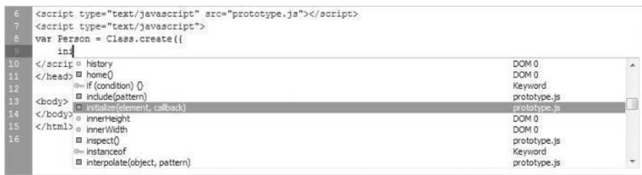
Figure 8-7. Dreamweaver's code introspection provides code hints for Prototype and other JavaScript libraries.
