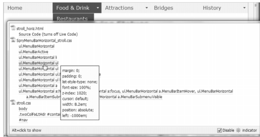
Figure 6-14. In Live view, the Code Navigator detects style rules that affect dynamically generated elements.
