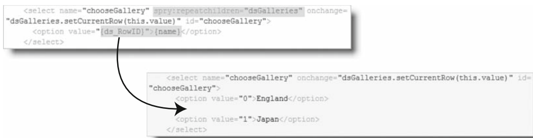
Figure 1-30. Live Code lets you see the HTML generated by JavaScript and server-side languages.
